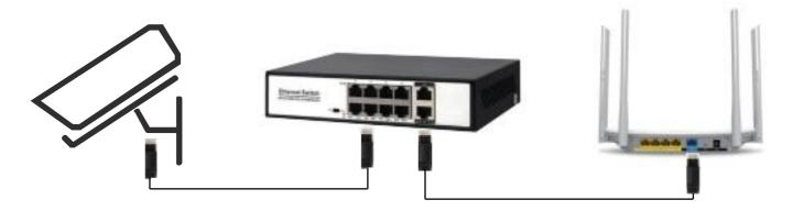
3. Install the camera to outside, POE Switch support 100meters(CAT5) max.
