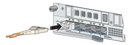
**Step 3** Connect the other end of the LC cable to a network device, such as a router or switch.
