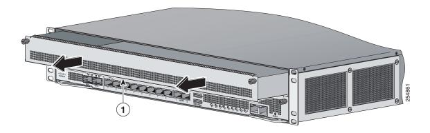
**Step 4** Install the IPS SSP by lining it up with the module slot making sure the ejection levers are extended.
