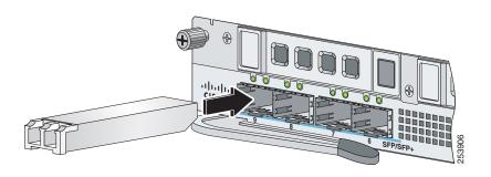
**Step 2** Connect one end of the LC cable to the SFP/SFP+.
