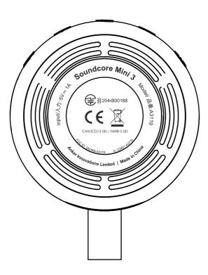
The Label's material is silk-screen, it cannot be easily erased. The size for the label is 40mm\*40mm
