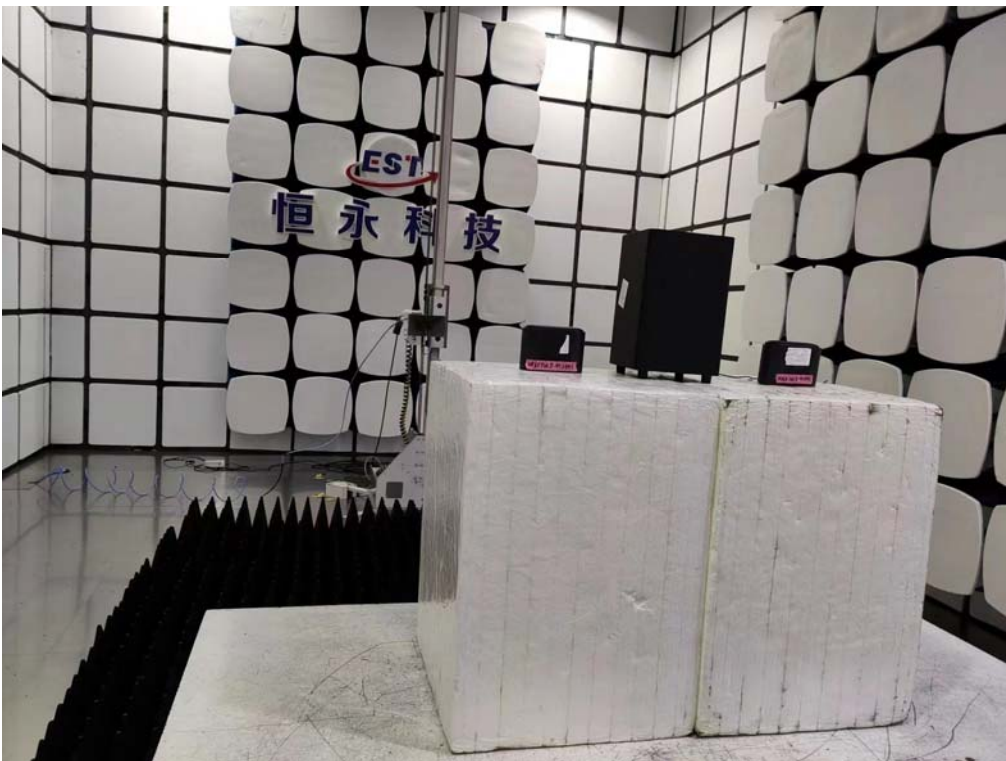
Radiated Test (Above 1GHz)
