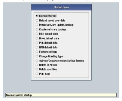
4. Select the "Install software update/backup" option to install an update on the system CompactFlash card from the user CompactFlash card or USB flash drive.
