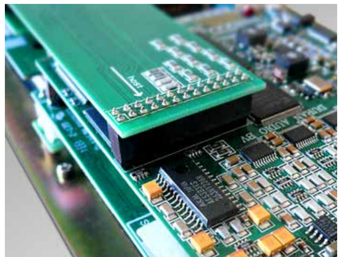
Integrated electronics module which combines powerful Digital Signal Processing with multi-channel class D Amplifiers
