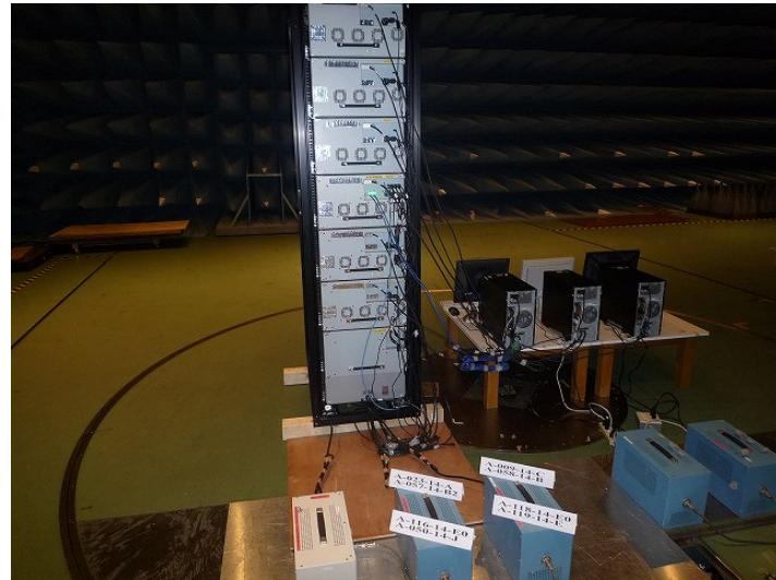
Spurious Emissions Measurement (Radiated)
