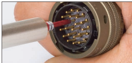
Typical application showing tool testing pin contacts.
