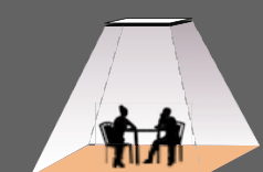
Mounted directly overhead is preferred and provides maximum coverage
