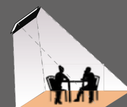
Angled mounting from the wall or ceiling is possible with the standard bracket, however the heating area is reduced
