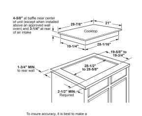
2" MIN. Clearance from cutout to nearest vertical wall or cabinet on right side of the unit below the 15" MIN clearance height. 30" MIN. Clearance from countertop to unprotected overhead surface See label next to nameplate for MIN, clearance to rear wall 15" MIN. height from countertop to nearest cabinet (including light rails) on both sides of 2" MIN. clearance cooktop to side wall from cut-out on the left of the unit
