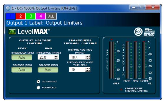
Shown as set for Control 47C/T at Low-Z ( $8\Omega$ ), listed for a Limiter Voltage of 23V RMS
