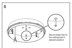
Position and fix the base to a suitable solid surface using screws supplied. Enter supply cable into the luminaire through a previously selected hole ensuring that the aperture is smooth or use a grommet where possible.
