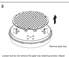
the position of the gear tray to align the hole in the keyhole slots
