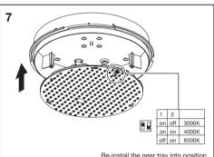
Re-install the gear tray into position
