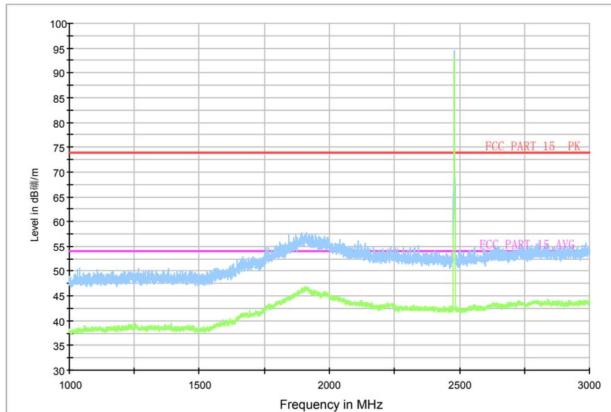
Fig.84. Radiated emission: 8DPSK, Channel 78, 1 GHz - 3 GHz
