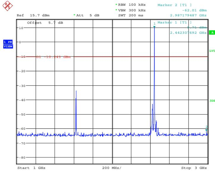
Fig.50. Conducted spurious emission: 8DPSK, Channel 39, 1GHz - 3GHz
