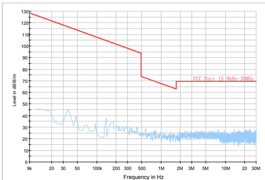
Fig.60. Radiated emission: GFSK, Channel 39, 9 kHz - 30 MHz
