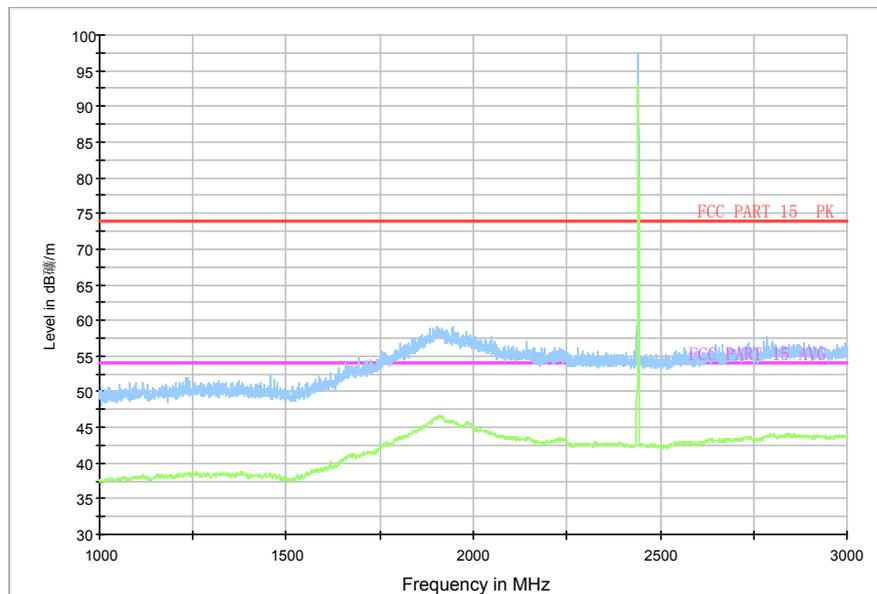
Fig.72. Radiated emission:  $\pi/4$  DQPSK, Channel 39, 1 GHz - 3 GHz
