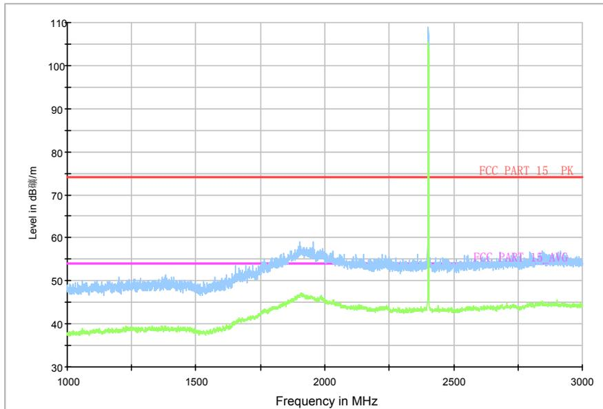
Fig.79. Radiated emission: 8DPSK, Channel 0, 1 GHz - 3 GHz
