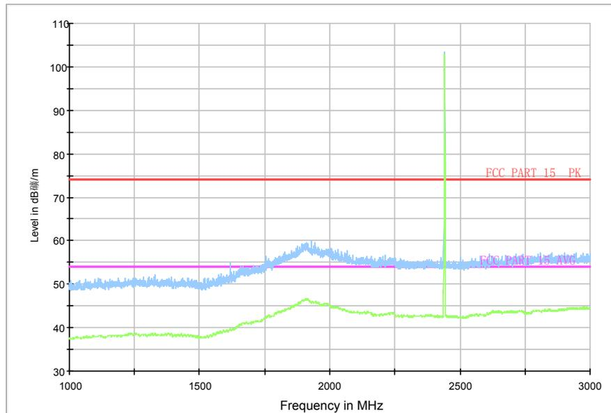
Fig.62. Radiated emission: GFSK, Channel 39, 1 GHz - 3 GHz
