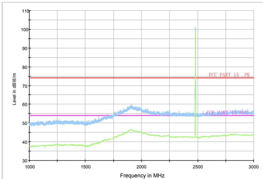
Fig.64. Radiated emission: GFSK, Channel 78, 1 GHz - 3 GHz
