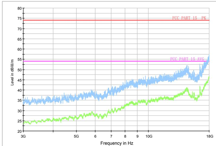
Fig.65. Radiated emission: GFSK, Channel 78, 3 GHz - 18 GHz
