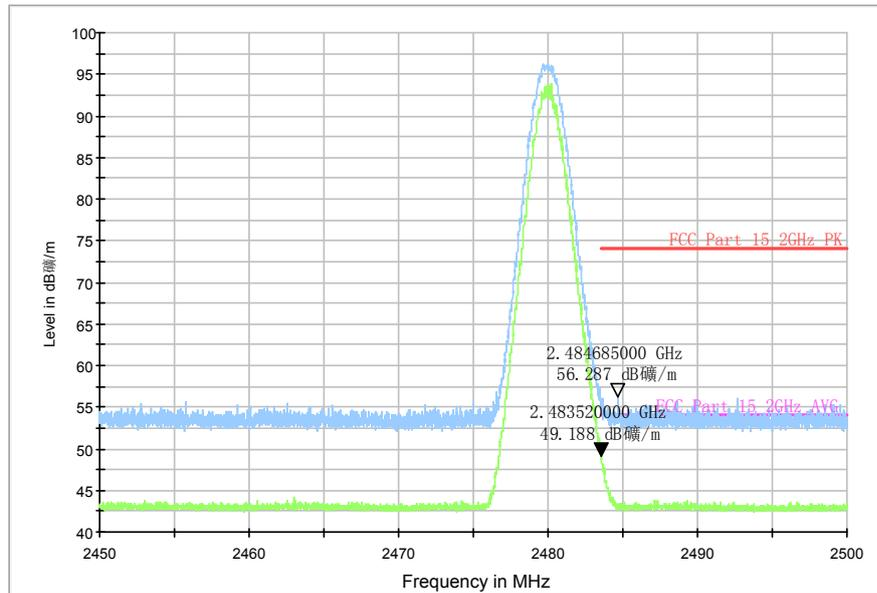
Fig.77. Radiated emission (Power):  $\pi/4$  DQPSK, high channel
