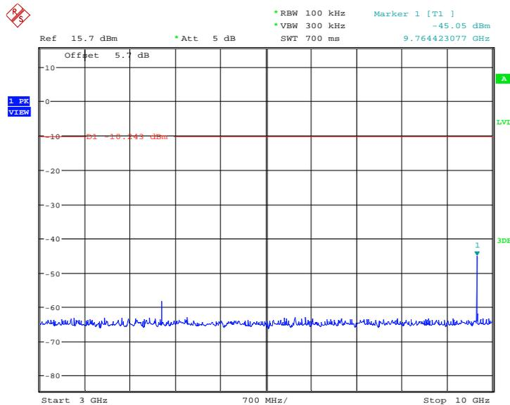
Fig.51. Conducted spurious emission: 8DPSK, Channel 39, 3GHz - 10GHz
