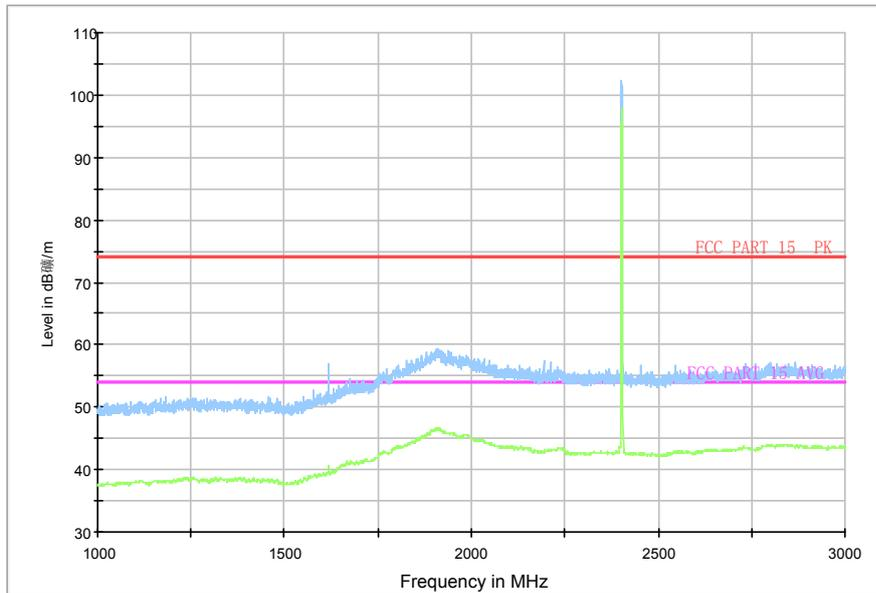
Fig.69. Radiated emission:  $\pi/4$  DQPSK, Channel 0, 1 GHz - 3 GHz
