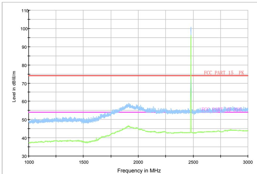
Fig.74. Radiated emission:  $\pi/4$  DQPSK, Channel 78, 1 GHz - 3 GHz
