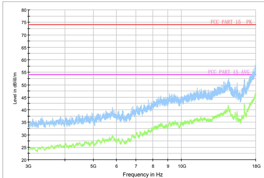
Fig.83. Radiated emission: 8DPSK, Channel 39, 3 GHz - 18 GHz
