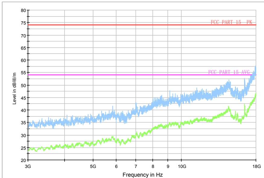
Fig.80. Radiated emission: 8DPSK, Channel 0, 3 GHz - 18 GHz
