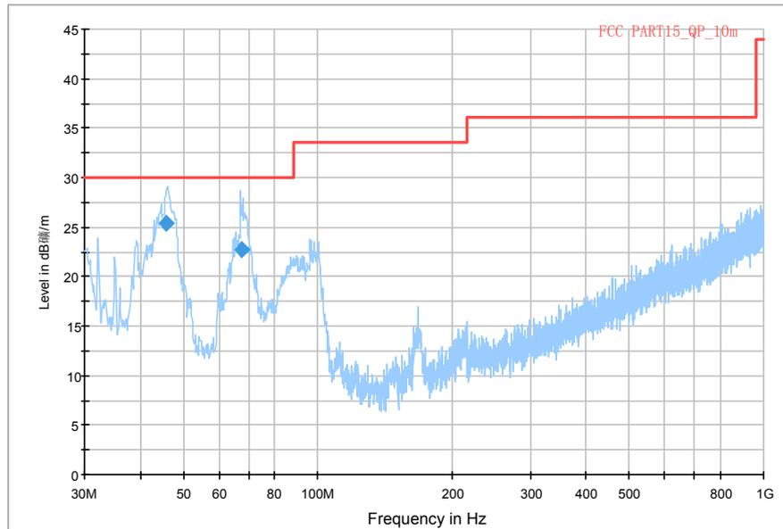
Fig.71. Radiated emission:  $\pi/4$  DQPSK, Channel 39, 30 MHz - 1 GHz
