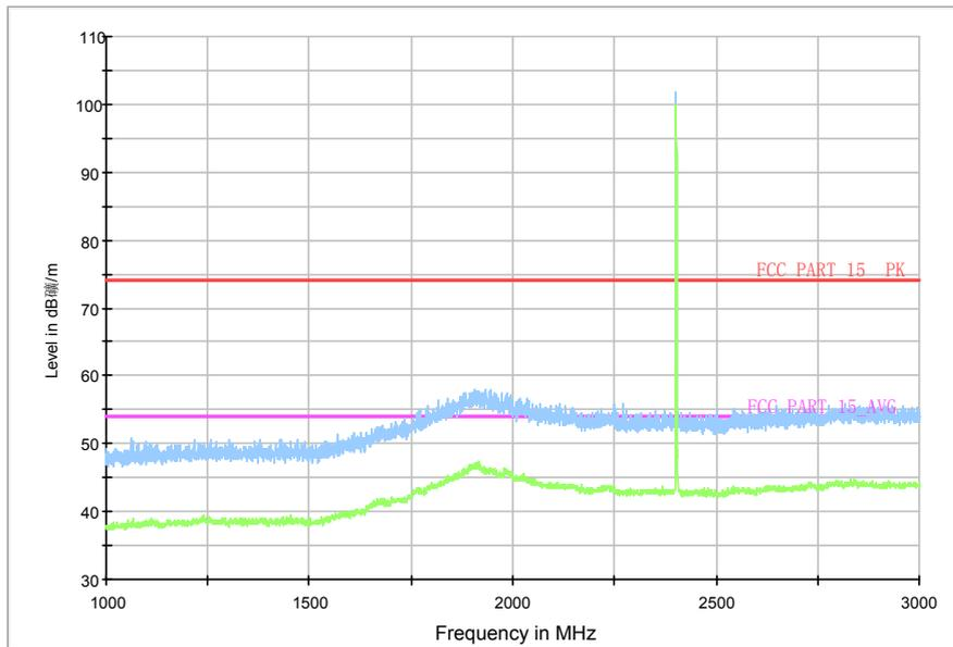
Fig.82. Radiated emission: 8DPSK, Channel 39, 1 GHz - 3 GHz
