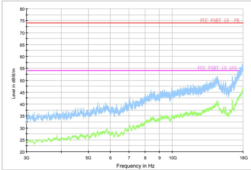
Fig.63. Radiated emission: GFSK, Channel 39, 3 GHz - 18 GHz
