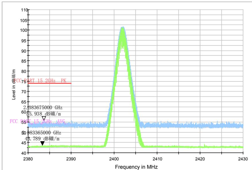
Fig.86. Radiated emission (Power): 8DPSK, low channel
