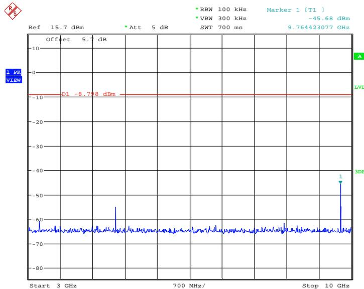
Fig.21. Conducted spurious emission: GFSK, Channel 39, 3GHz – 10GHz
