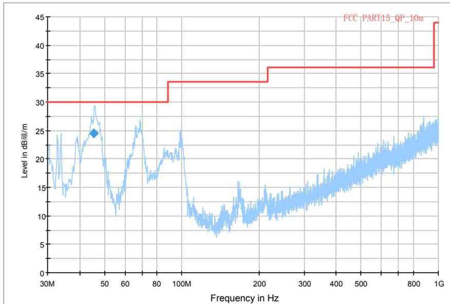
Fig.81. Radiated emission: 8DPSK, Channel 39, 30 MHz - 1 GHz
