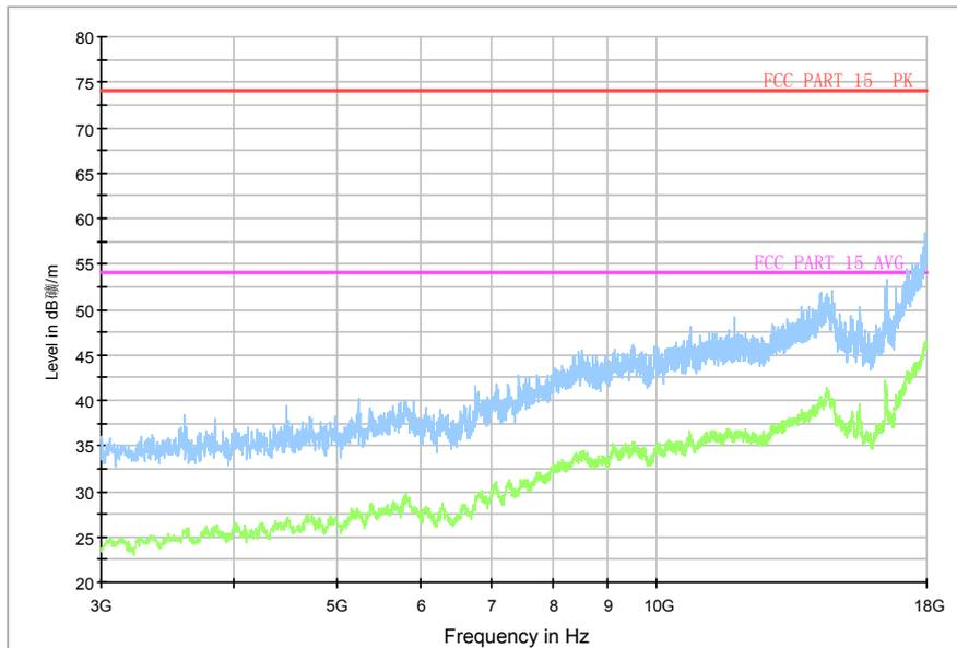
Fig.70. Radiated emission:  $\pi/4$  DQPSK, Channel 0, 3 GHz - 18 GHz
