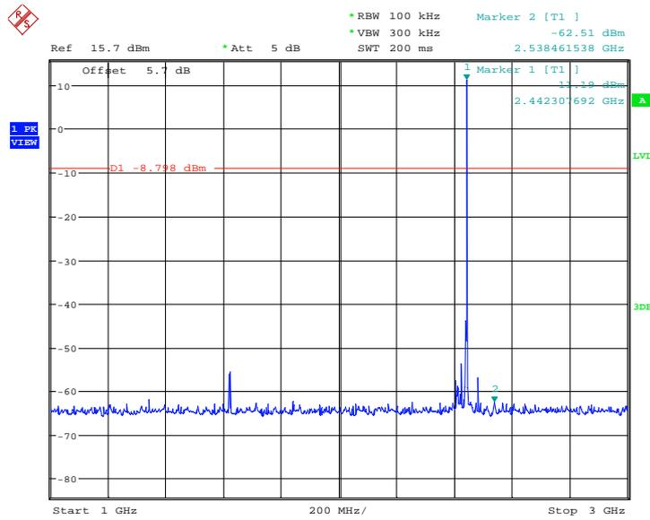
Fig.20. Conducted spurious emission: GFSK, Channel 39, 1GHz – 3GHz
