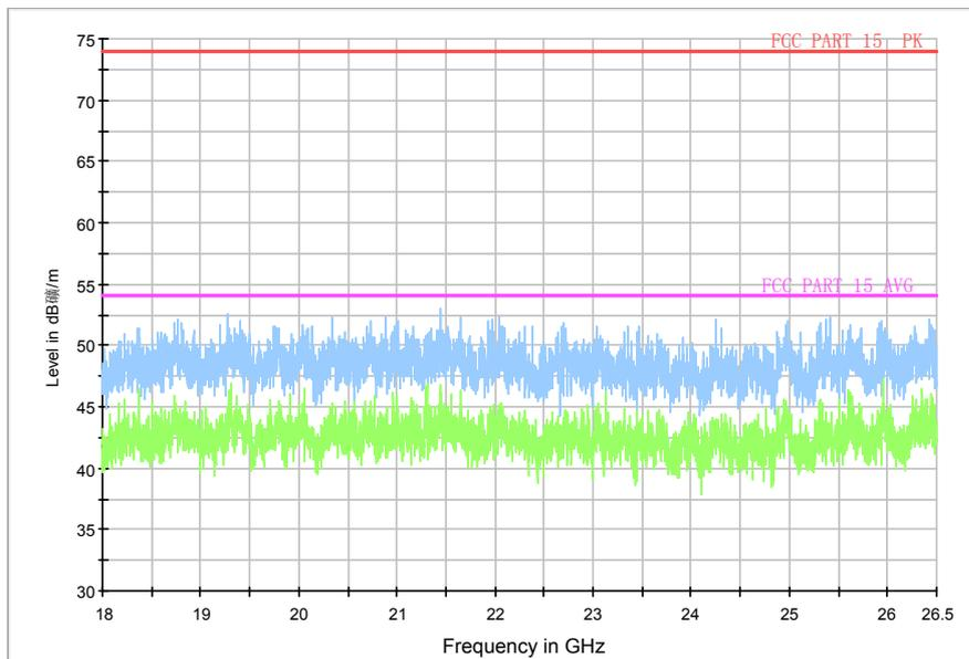
Fig.88. Radiated emission: 8DPSK, 18 GHz - 26 GHz
