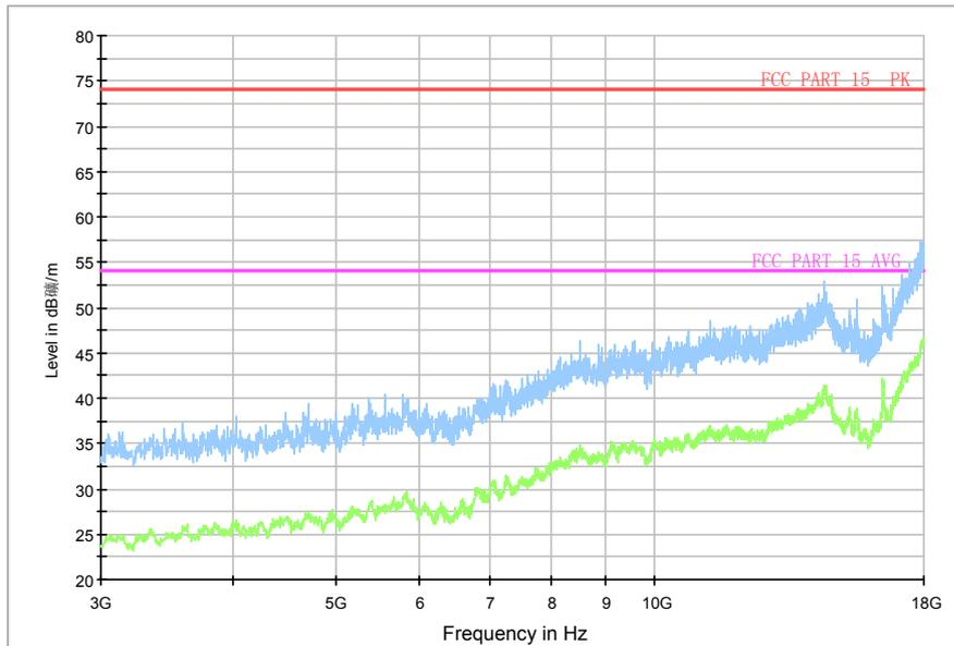
Fig.85. Radiated emission: 8DPSK, Channel 78, 3 GHz - 18 GHz
