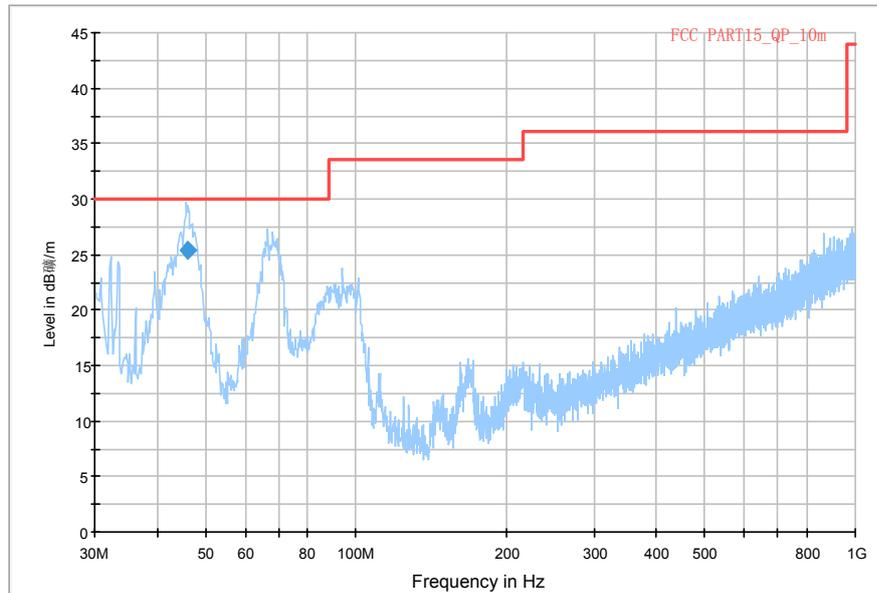
Fig.61. Radiated emission: GFSK, Channel 39, 30 MHz - 1 GHz
