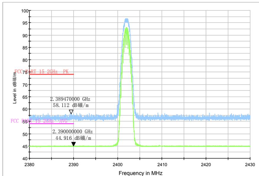
Fig.76. Radiated emission (Power):  $\pi/4$  DQPSK, low channel
