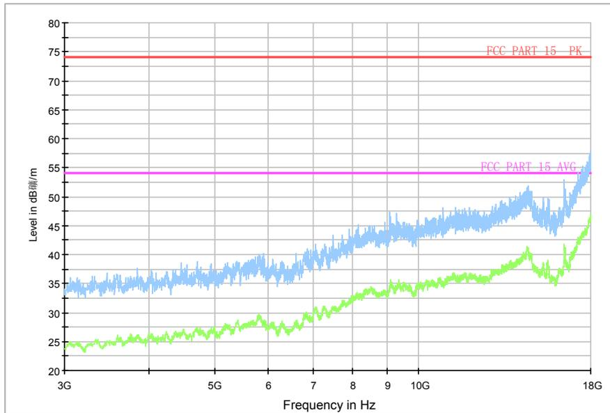
Fig.59. Radiated emission: GFSK, Channel 0, 3 GHz - 18 GHz
