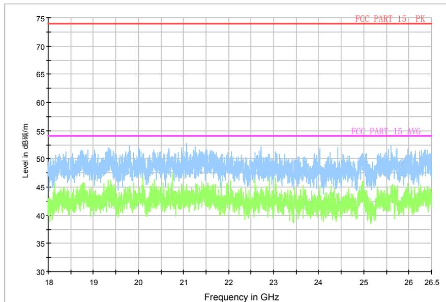
Fig.68. Radiated emission: GFSK, 18 GHz - 26 GHz
