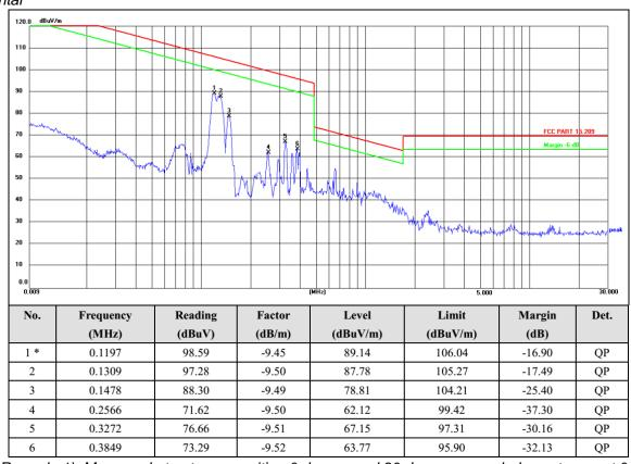
Remark: 1). Measured at antenna position 0 degree and 90 degree, recorded worst case at 0 degree. 2). Margin=Reading level + Factor- Limit
