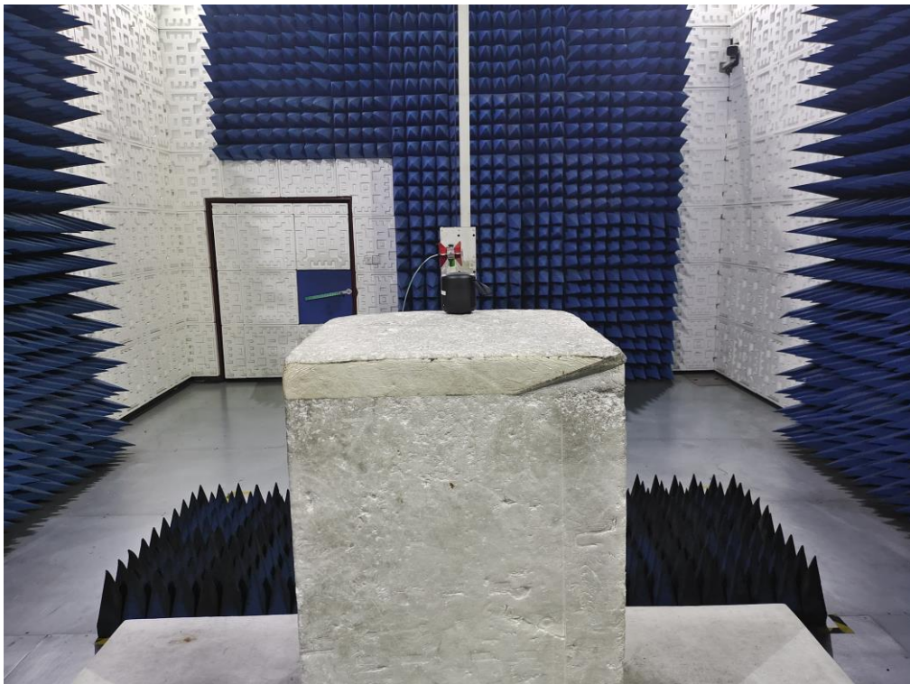
RADIATED EMISSION TEST SETUP ABOVE 1GHz
