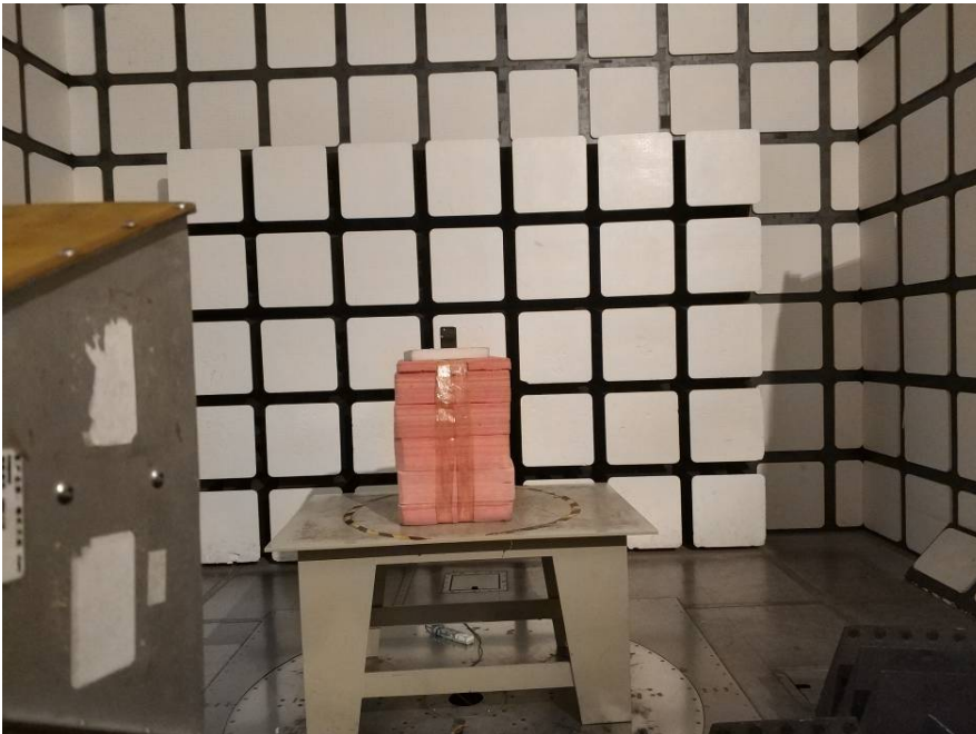
Radiated Emissions View (Above 1 GHz)
