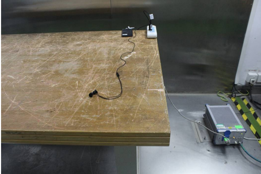
Conducted Emissions - Front View
