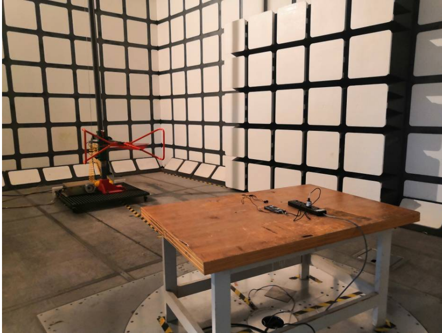
Radiated Emissions View (Below 1 GHz)
