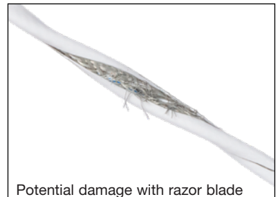
Potential damage with razor blade
