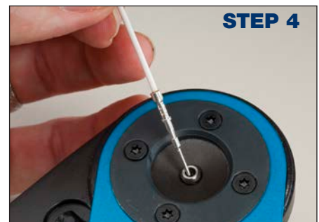
REMOVE TERMINATED WIRE ASSEMBLY
