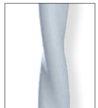
LEFT HAND LAY "S" DIRECTION
