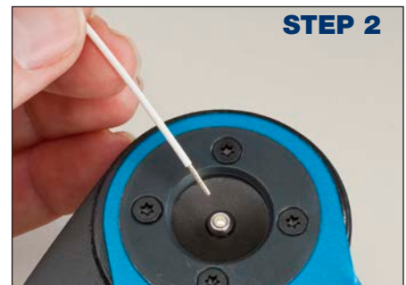
INSERT PRE-STRIPPED WIRE
