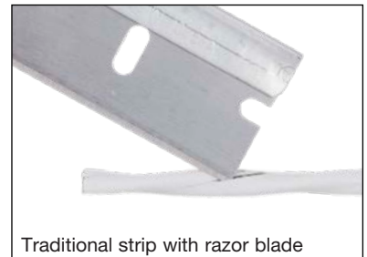
Traditional strip with razor blade
