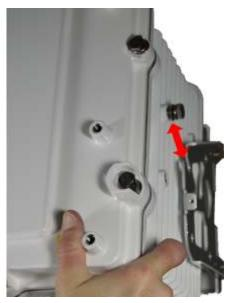
1. Mount the CGR to the mounting bracket by sliding the mounting bolt in the top front position on each side of the CGR into the corresponding slot on the mounting bracket.
