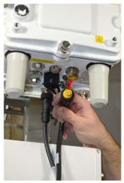
5. Connect the 6-pin female end of the PLC signal cable to the male PLC signal bulkhead connector on the CGR.
