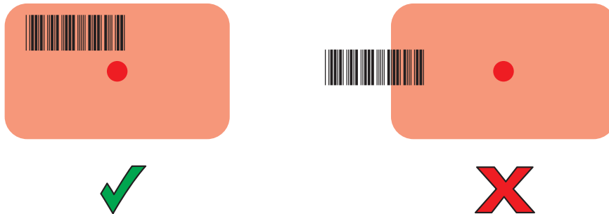
Figure 32 DS3678 Pick List Mode with Multiple Barcodes in Aiming Pattern
