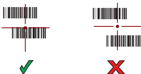
Figure 25 RS507/RS507X Pick List Mode with Multiple Barcodes in Aiming Pattern
