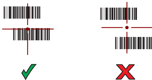
Figure 27 RS6000 Pick List Mode with Multiple Barcodes in Aiming Pattern
