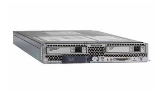
The enterprise-class Cisco UCS B200 M5 blade server extends the capabilities of the Cisco UCS portfolio in a half-width blade form factor. The Cisco UCS B200 M5 blade server harnesses the power of the latest Intel Xeon processor scalable family CPUs with up to 3072GB of RAM (using 128GB DIMMs), two solid-state drives (SSDs) or HDDs, and up to 80Gbps throughput connectivity.
