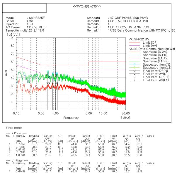
Note 1) Two graphs measured for both Live(L1) and Neutral(N) of the LISN are combined into one graph.
