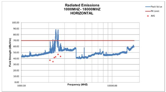
Figure 6.Radiated Emissions Above 1 GHz Horizontal
