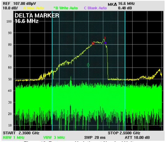
Figure 13. Frequency Variation at Nominal Voltage
