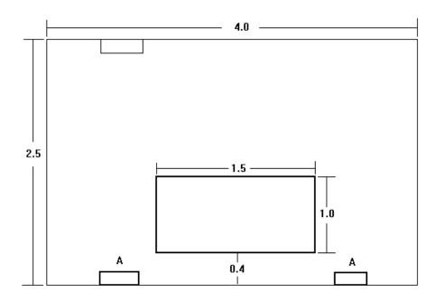
Figure 2. Power Line Emissions Disturbance Measurement Facility Diagram
