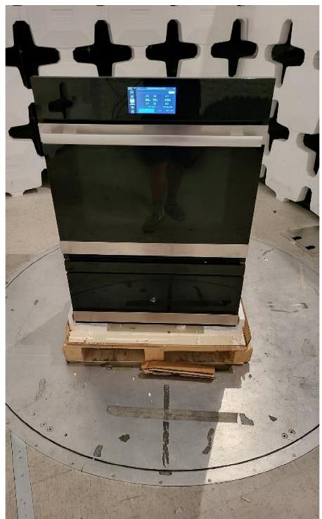
Figure 9. Photograph of Radiated Emissions Test Configuration, Close-Up
