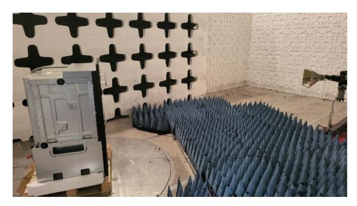
Figure 12. Photograph of Radiated Emissions Test Configuration, above 1000 MHz
