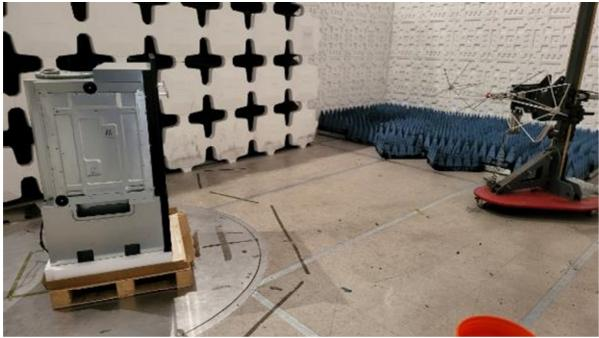
Figure 10. Photograph of Radiated Emissions Test Configuration, 30 - 200 MHz
