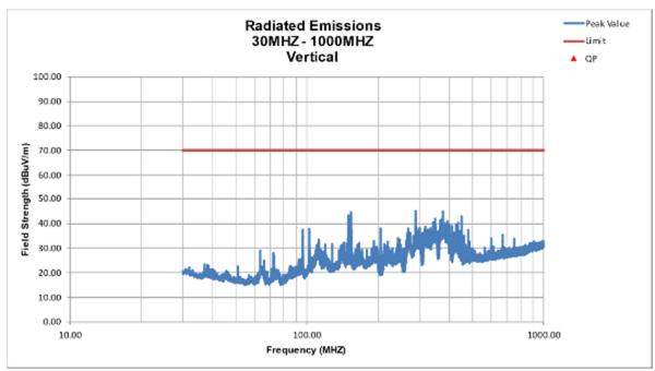
Figure 5. Radiated Emissions Below 30-1000 MHz Vertical
