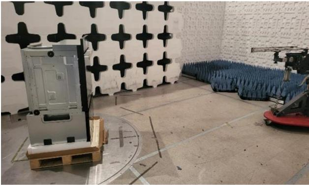
Figure 11. Photograph of Radiated Emissions Test Configuration, 200 - 1000 MH
