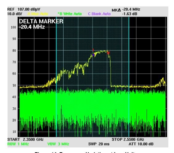
Figure 14. Frequency Variation at Low Voltage
