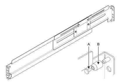
Loosen the two screws attached to the side of rail (A in Figure 3-7) and confirm that the brackets at the front and rear can slide.
