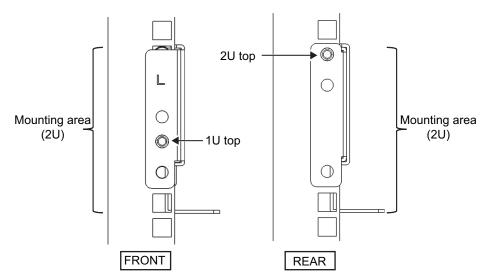
Figure 3-30 Attaching the Rails: Fixing Point of the Screw
