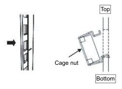
b. Insert the hook at the tip of the supplied cage nut attachment tool through a cage nut attachment hole from the front, and engage it with the hook at the other end of the cage nut.
