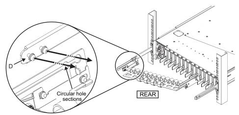
b. Slide the cable support all the way in, and tighten the four screws (C in Figure 3-39).
