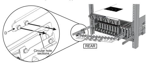
b. Slide the cable support all the way in, and tighten the four screws (C in Figure 3-18).
