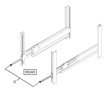
Figure 3-13 Securing a Cable Support Fixing Bracket and Rail
