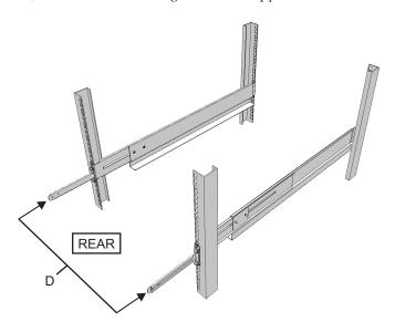
Figure 3-34 Securing a Cable Support Fixing Bracket and Rail
