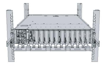
Figure 3-42 PCI Expansion Unit Mounting Completed
