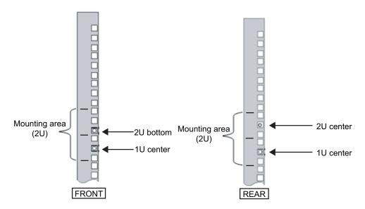
a. Attach cage nuts from the inside of the rack. Orient the hooks of the cage nut vertically.
