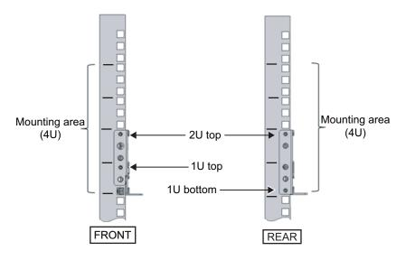
Figure 3-9 Attaching the Rails: Fixing Point of the Screw
