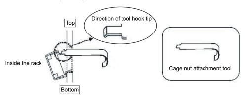
c. Pull the tool forward to attach the cage nut.
