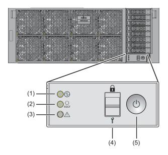
Table 2-13 LEDs and Switches on the Operation Panel
