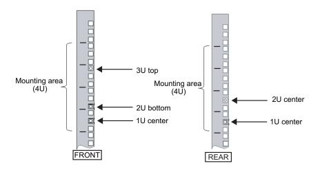
a. Attach cage nuts from the inside of the rack.
