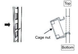
b. Insert the hook at the tip of the supplied cage nut attachment tool through a cage nut attachment hole from the front, and engage it with the hook at the other end of the cage nut.
