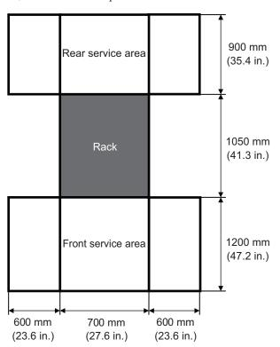
Figure 2-3 Example of Service Areas for the PCI Expansion Unit (Top View)
