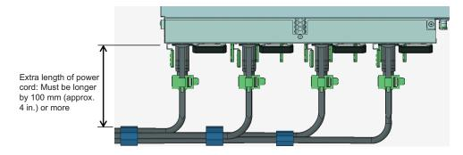
Figure 4-8 Reference: Example of Active Maintenance of a Power Supply Unit
