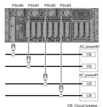
Figure 2-5 Power Supply Systems With Dual Power Feed
