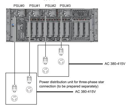
Figure 2-7 Power Supply System With Three-Phase Power Feed (Delta Connection)
