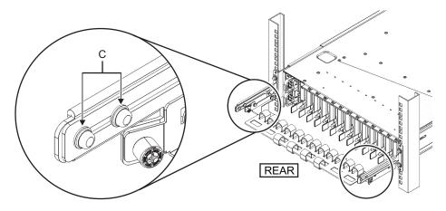
**Note -** If the dimension between the front and rear columns of the rack is less than 740 mm, secure the cable support without sliding it all the way in. The fixing point varies depending on the dimension between the front and rear columns of the rack. Based on Figure 3-40, align the scale marks (E in Figure 3-40) (spacing: 10 mm) on the cable support with the screws (F in Figure 3-40) of the fixing brackets to secure the cable support.
