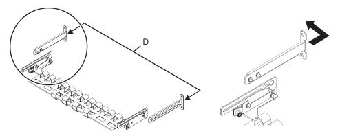
c. From the rear of the rack, secure the rails and cable support fixing brackets (D) with two M6 screws to the rear supporting columns of the rack. The fixing points are 1U center and 2U center.
