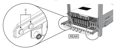
**Note** - If the dimension between the front and rear columns of the rack is less than 740 mm, secure the cable support without sliding it all the way in. The fixing point varies depending on the dimension between the front and rear columns of the rack. Based on Figure 3-19, align the scale marks (E in Figure 3-19) (spacing: 10 mm) on the cable support with the screws (F in Figure 3-19) of the fixing brackets to secure the cable support.
