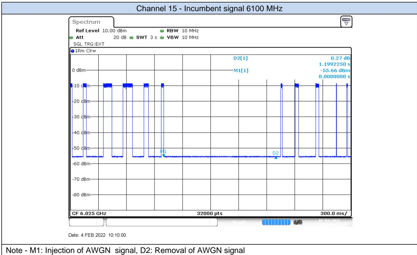
Note - M1: Injection of AWGN signal, D2: Removal of AWGN signal
