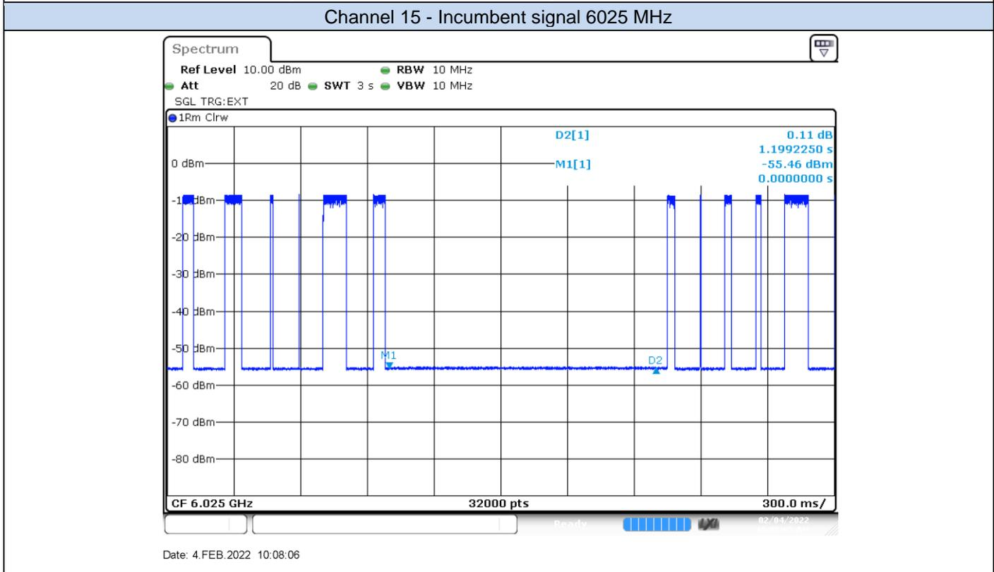
Note - M1: Injection of AWGN signal, D2: Removal of AWGN signal
