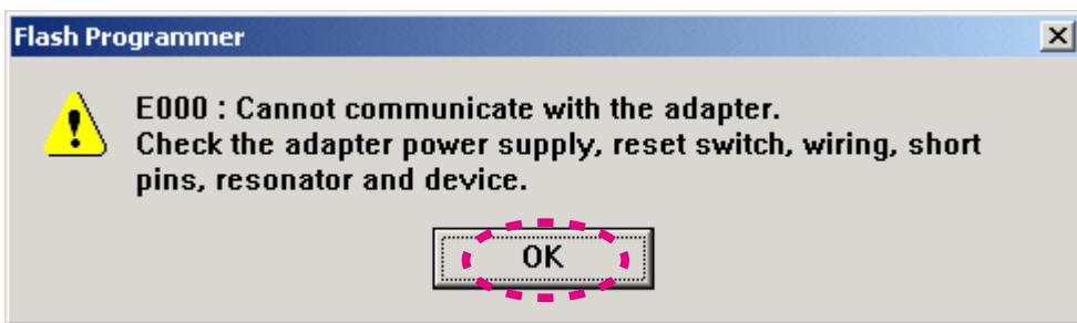
**NOTE** : Since Flash Programmer communicates with the unit automatically, the above dialog box appears when it fails in communication.
