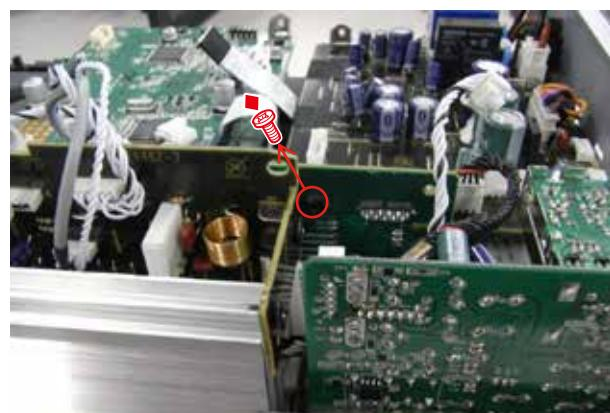
(4) Disconnect the connector wire, then remove the screws.
