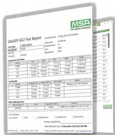
GALAXY GX2 and MSA Link Pro Software allows for automated calibration, bump testing and fleet management
