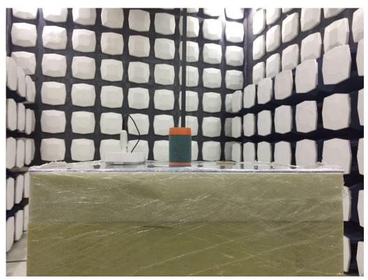
Front View of Radiated Emissions above 1GHz
