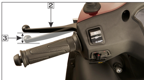
(2) Integrated brake lever (3) Free play: 20-30 mm
