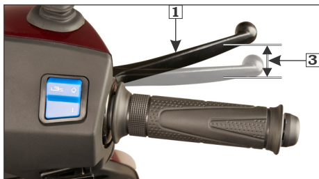
(1) Front brake lever (3) Free play: 20-30 mm
