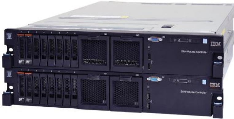
Figure 14 IBM SAN Volume Controller
