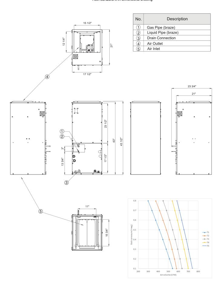
Samsung Multi-Position Air Handler, Single Zone Duct, Split System AC018BXADCH/AA Dimensional Drawing
