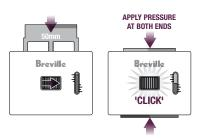
Adjust the Razor™ to the setting in the table below for your Breville espresso machine. This is a starting point for your dose height.
