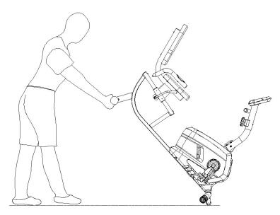
Hold the **Rear Stabilizer (No. 3)** and lift the bike until wheels on the **Front Stabilizer (No. 9)** touch the ground. Now you can wheel the bike to the desired location.
