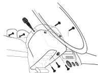
2. Place the ring of the antenna around the vehicle's ignition switch as shown below.
