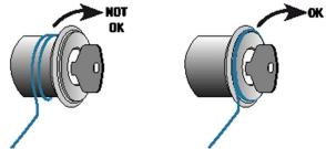
Fix and tape the ring around the ignition, excess cable can be taped together but may not be turned around (one rotation maximum). When using the ring method for installing the ACCM the ring MUST be taped in front of the factory receiver ring. It CAN NOT be on top of, or behind the factory receiver ring. See illustration above. The antenna cable must follow existing steering column cables to avoid rupture while closing the shroud or moving the steering wheel.
