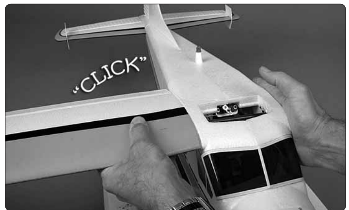
❑ 2. Guide the wires from the right wing into the fuselage, then slide the wing joiner tube and the flap pushrod wire through the corresponding holes. Also guide the flap pushrod wire into the screw-lock connector on the flap servo. Guide the joiner tube through the hole in the left side of the fuselage, then tightly "CLICK!" the wing onto the wing clips.
