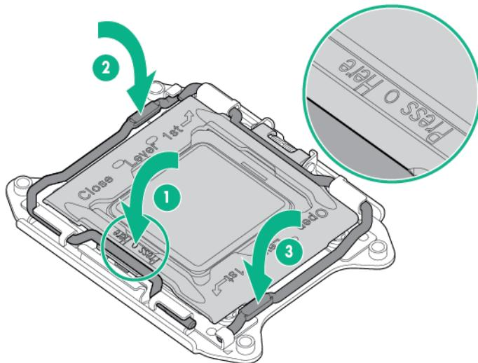
8. Install the processor socket cover on the failed system board.
