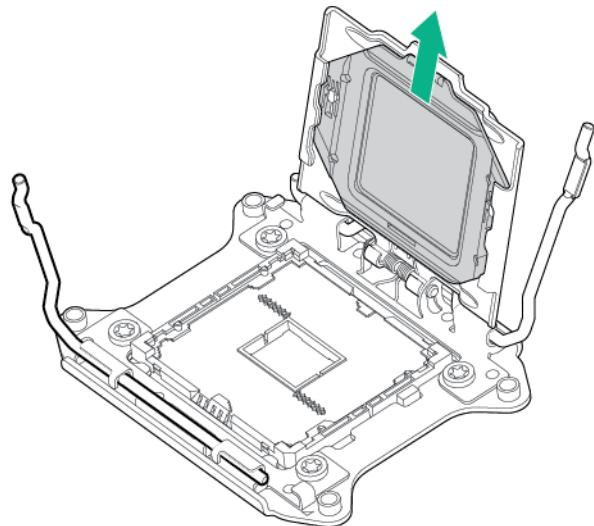
5. Install the processor. Verify that the processor is fully seated in the processor retaining bracket by visually inspecting the processor installation guides on either side of the processor. **THE PINS ON THE SYSTEM BOARD ARE VERY FRAGILE AND EASILY DAMAGED.**
