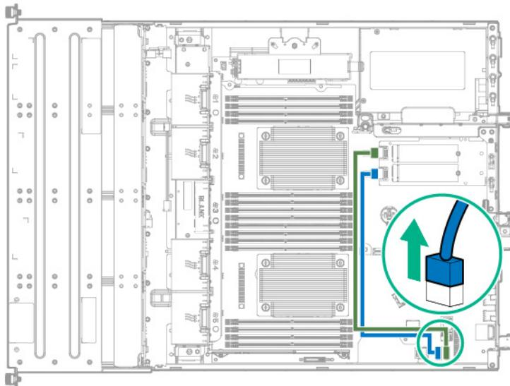
6. Remove the PCI riser cage ("Remove the PCI riser cages" on page 32).
