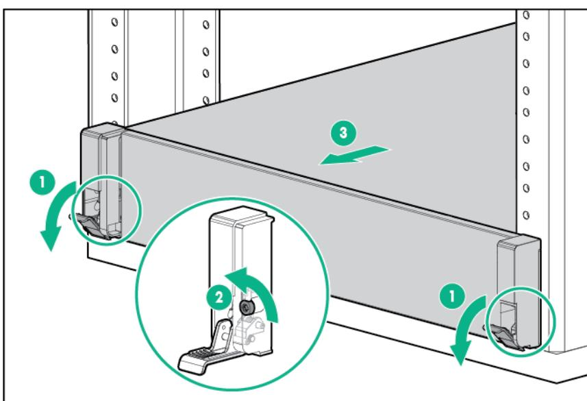
4. After performing the installation or maintenance procedure, slide the server back into the rack, and then press the server firmly into the rack to secure it in place.
