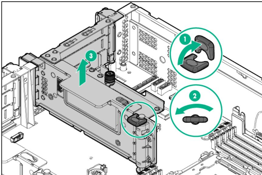
7. If an expansion board is installed in the PCI riser cage, remove the board ("Expansion board" on page 59).
