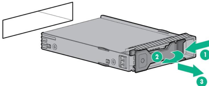
6. Remove the drive from the carrier.
