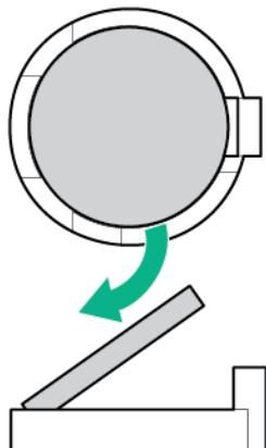
2. If the battery socket design has a plastic outer lip to secure the battery, insert the battery with the "+" side facing up underneath the outer lip of the socket, and then press the battery down to secure it in place.
