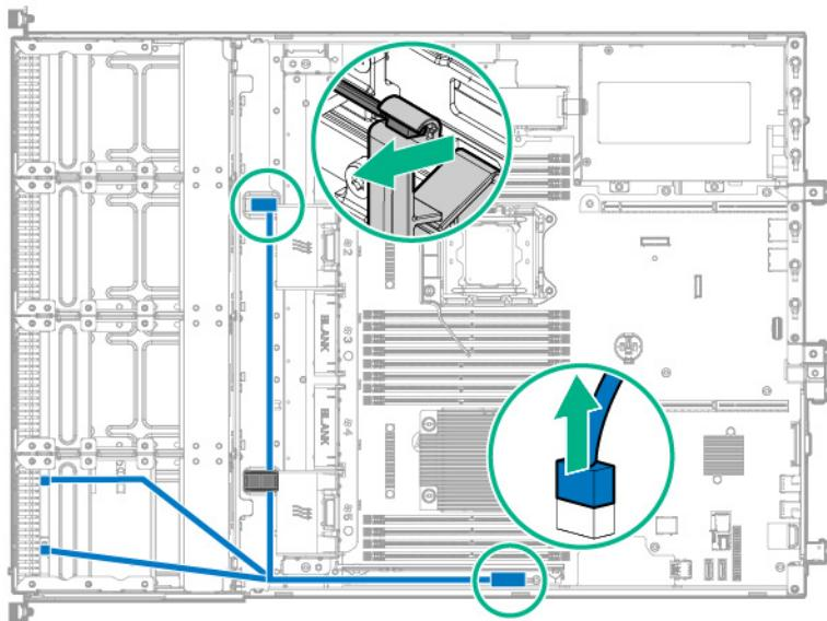
— Front I/O cabling disconnection in an SFF chassis
