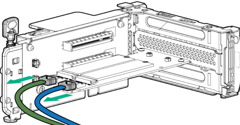
8. Remove the M.2 SSD enablement board.
