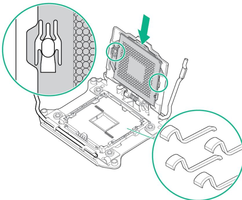
⚠ **CAUTION:** Do not press down on the processor. Pressing down on the processor may cause damage to the processor socket and the system board. Press only in the area indicated on the processor retaining bracket.
