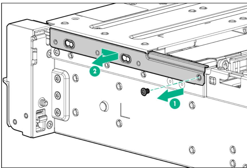
9. Remove the right quick-release latch rack ear assembly.
