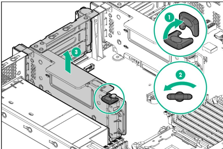
8. If expansion boards with internal cabling are installed on the PCI riser cage, disconnect all internal cables from the expansion boards to completely remove the cage from the server.
