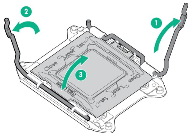
**CAUTION: THE PINS ON THE SYSTEM BOARD ARE VERY FRAGILE AND EASILY DAMAGED.** To avoid damage to the system board, do not touch the processor or the processor socket contacts.
