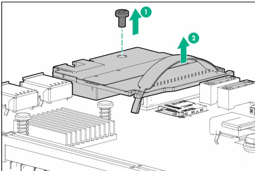
To replace the component, reverse the removal procedure. After installing the new dedicated iLO management module, enable the dedicated iLO connector ("Enabling the dedicated iLO management module" on page 66).
