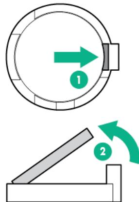
8. If the system battery is secured by a plastic outer clip, do the following:
