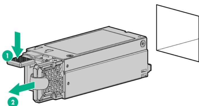
To replace the component, reverse the removal procedure.
