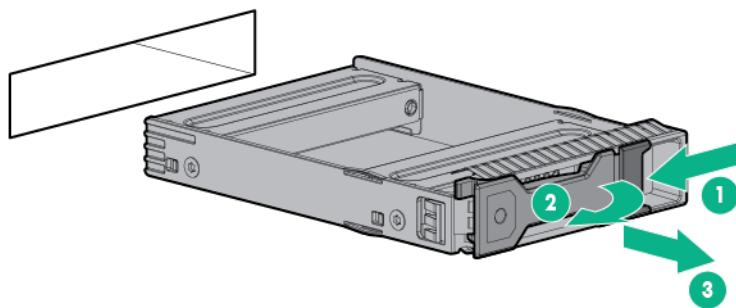
To replace the component, slide the component into the bay until it clicks.
