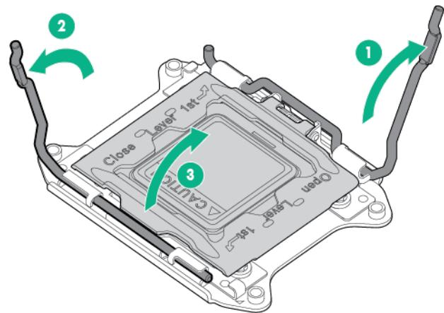
4. Remove the clear processor socket cover. Retain the processor socket cover for future use.
