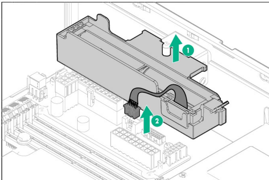
6. Remove the Smart Storage Battery from its holder.
