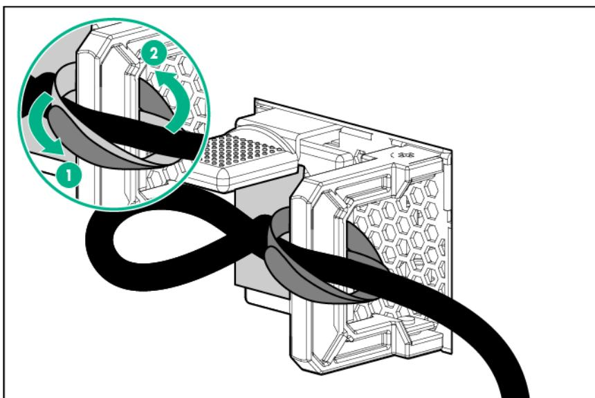
4. Disconnect the power cord from the power input module.
