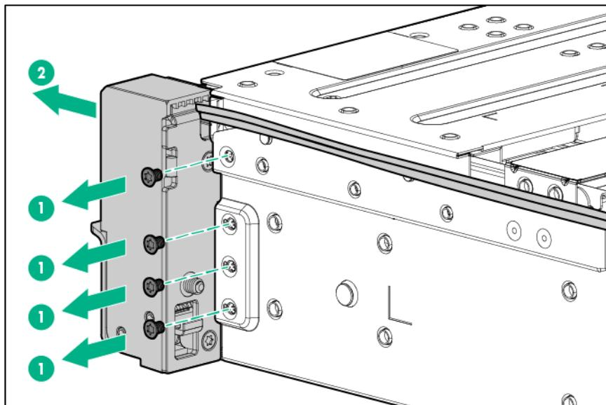
10. Remove the left quick-release latch rack ear.
