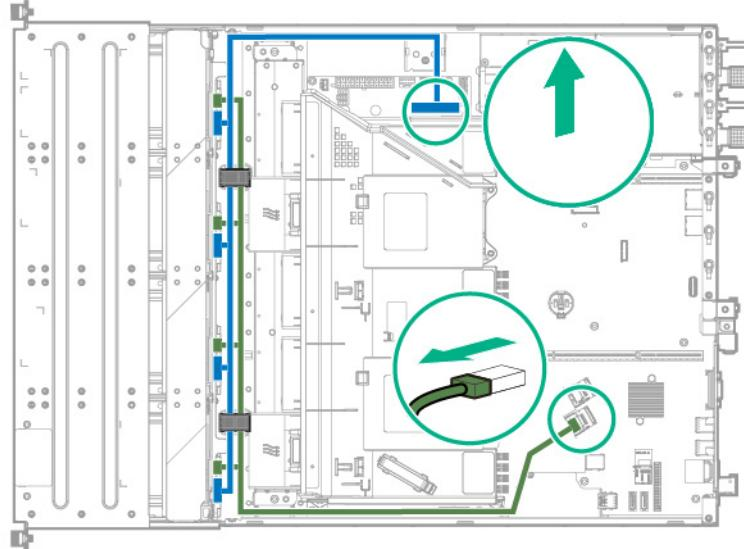
— 8-bay LFF non-hot-plug drive cable disconnections
