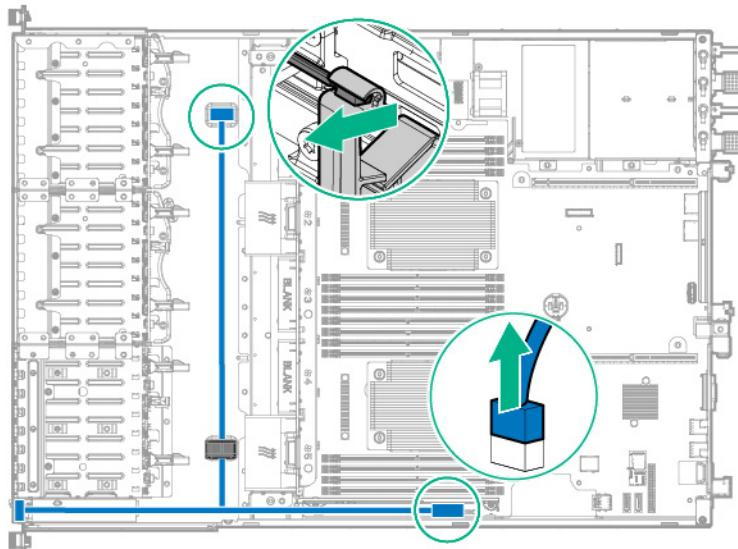
7. Remove the front I/O assembly from the chassis:
