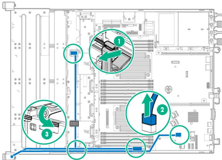
8. Remove the cable cover behind the right quick-release latch rack ear.
