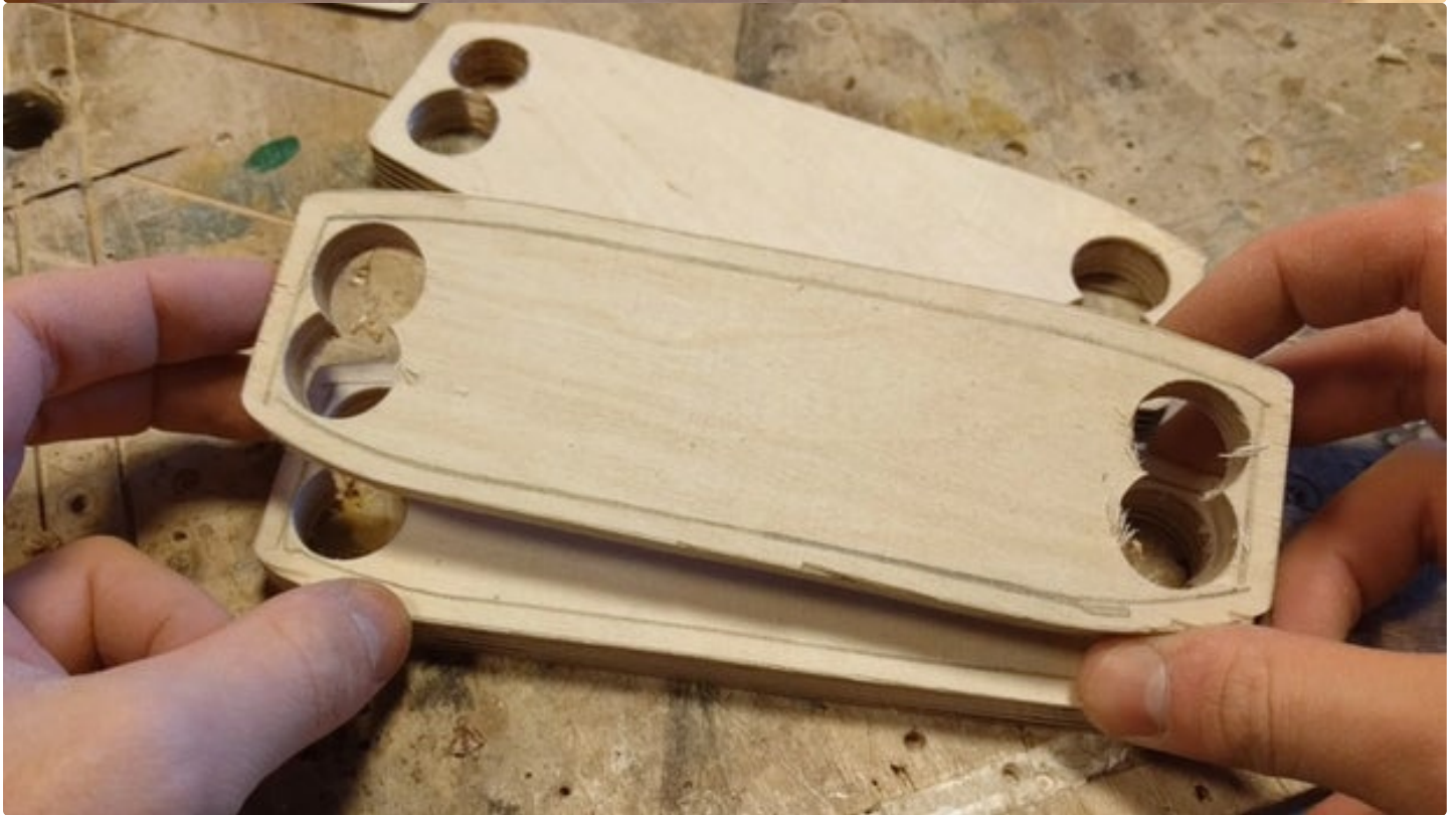
Drilling out the inside corners
