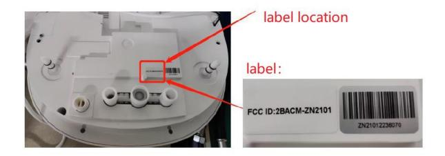
The label is attached to the bottom of the device with a permanent adhesive.
