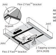
Align the edge of Flex-Z Fast™ with the edge of the ceiling opening on the side where the adapter will be installed.
