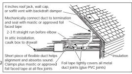
around the ducts can reduce energy loss and inhibit mold growth. Fans installed with existing ducts may not achieve their rated air flow.
