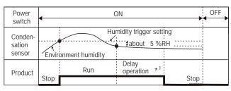
\* 1 The product will continue to run for about 20 minutes after the sensor detects that the humidity is ~5 % RH lower than the humidity setting before stopping.
