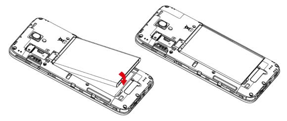
• Align the contacts of the battery with the contacts in the phone.
