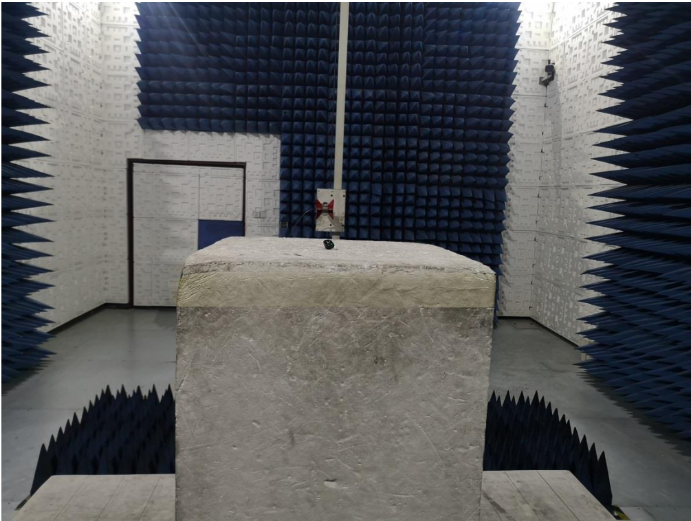
RADIATED EMISSION TEST SETUP ABOVE 1GHz
