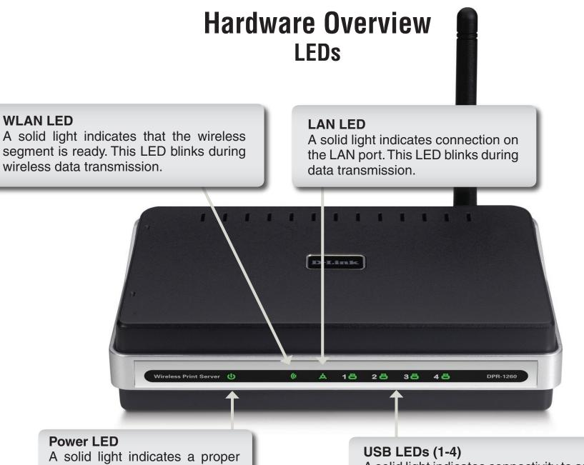
A solid light indicates connectivity to an USB printer or scanner.
