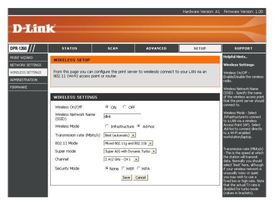
Compression, and Dynamic Turbo. This setting is backwards compatible with non-Turbo (legacy) devices. Dynamic Turbo mode is only enabled when all devices on the wireless network are Super G with Dynamic Turbo enabled.
