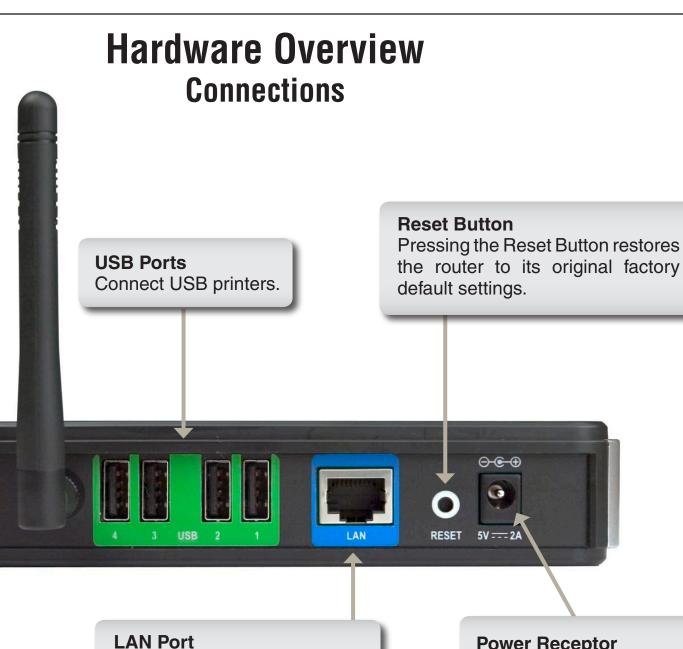
Connect to a network using an Ethernet cable.
