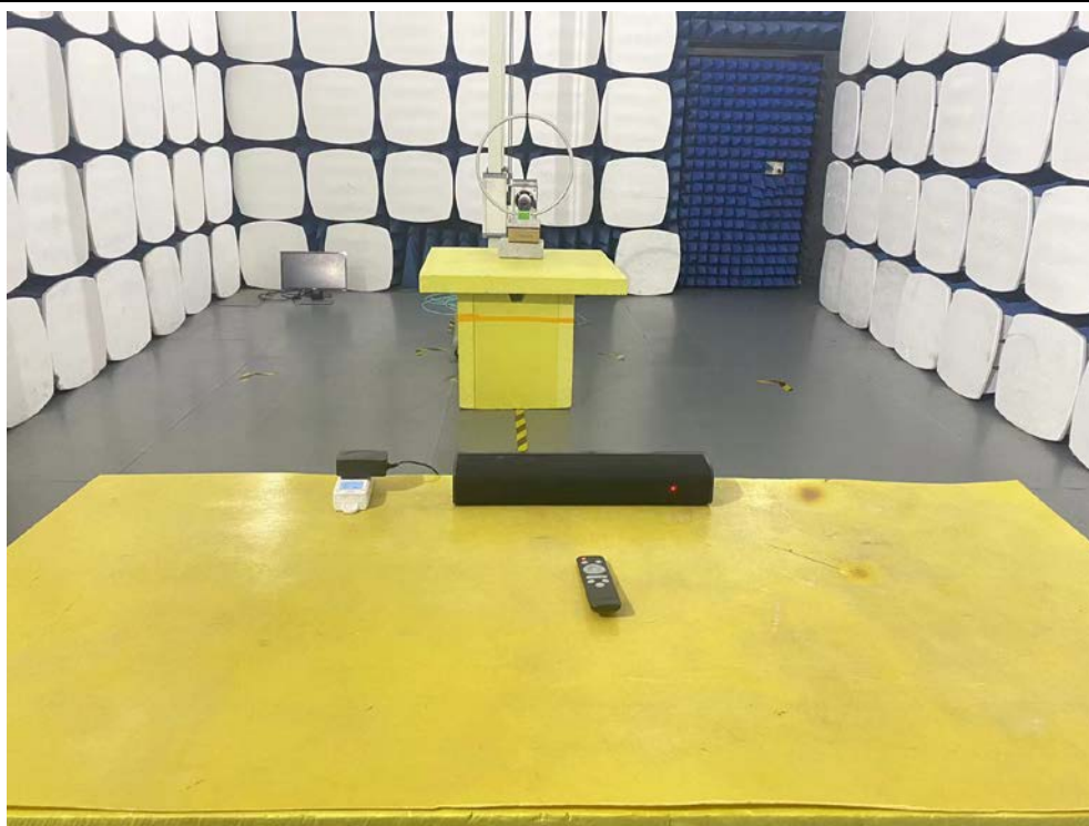
Radiated emission Test Setup (30MHz~1GHz)
