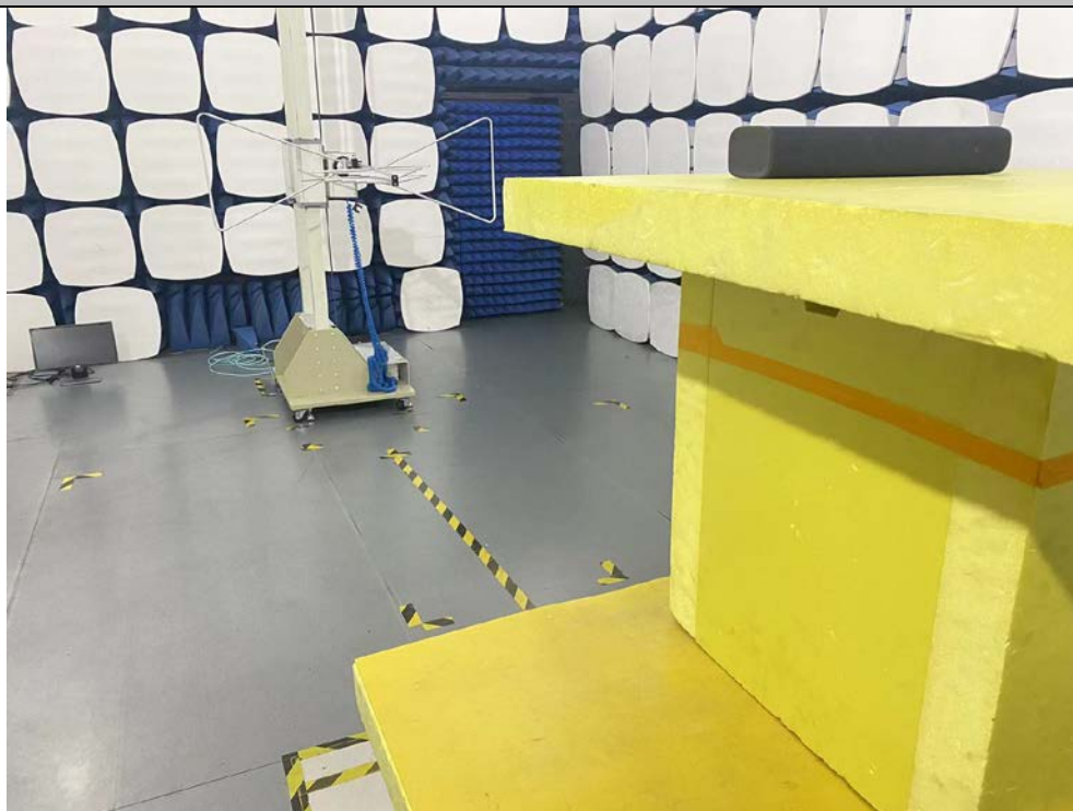
Radiated emission Test Setup (30MHz~1GHz)
