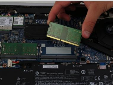
Once the side gates are removed the stick of RAM will pop up and you can pull it out.
