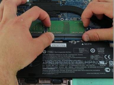
Using your fingers, remove the clips on the sides of the sticks of RAM by pulling up and towards you.
