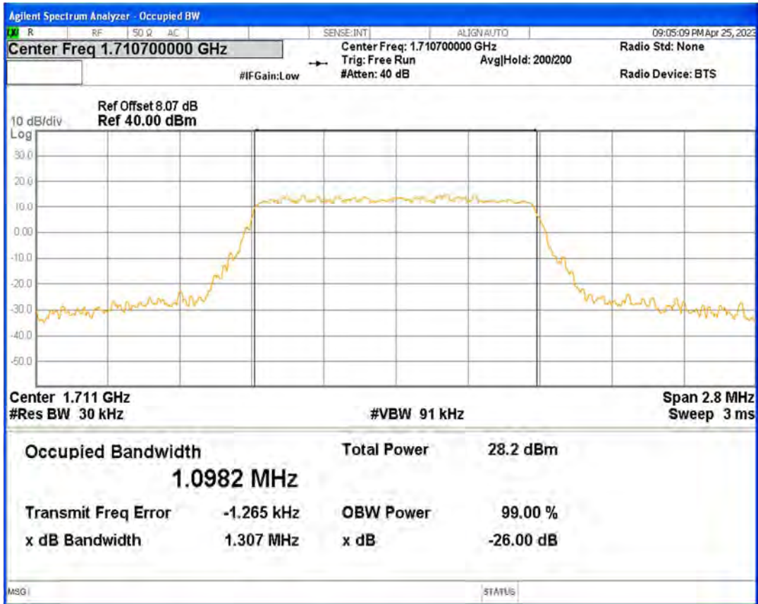
Band4 16QAM BW=1.4MHz Channel=20175 RB Size=6 Position=#0
