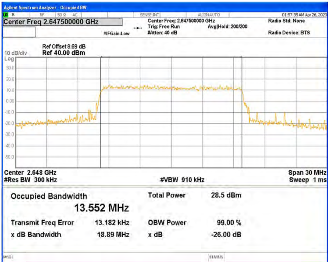
Band41(2555-2655) 16QAM BW=20MHz Channel=40340 RB Size=100 Position=#0
