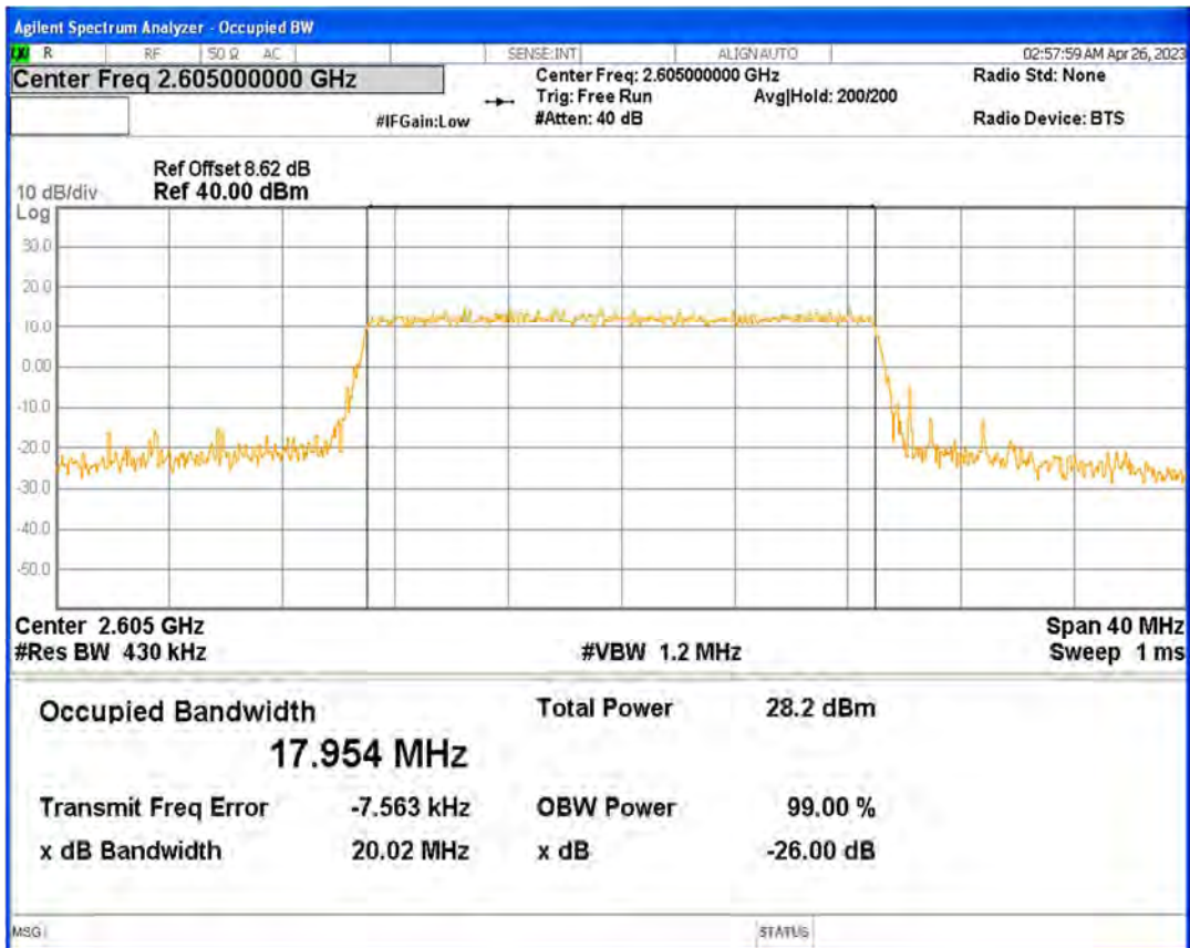
Band41(2555-2655) 16QAM BW=20MHz Channel=41140 RB Size=100 Position=#0
