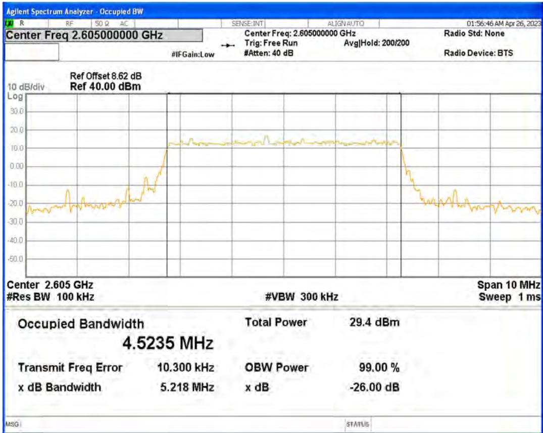
Band41(2555-2655) QPSK BW=5MHz Channel=41215 RB Size=25 Position=#0
