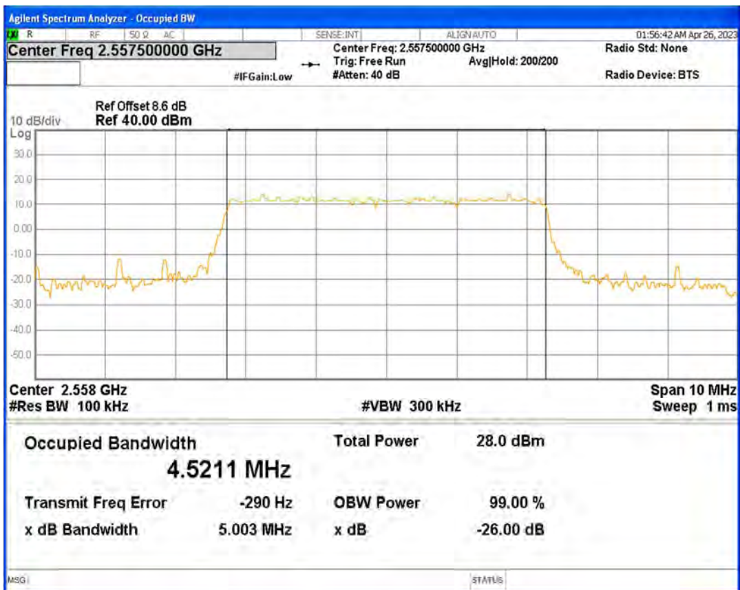
Band41(2555-2655) 16QAM BW=5MHz Channel=40740 RB Size=25 Position=#0
