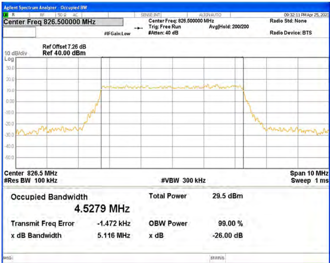
Band5 QPSK BW=5MHz Channel=20525 RB Size=25 Position=#0
