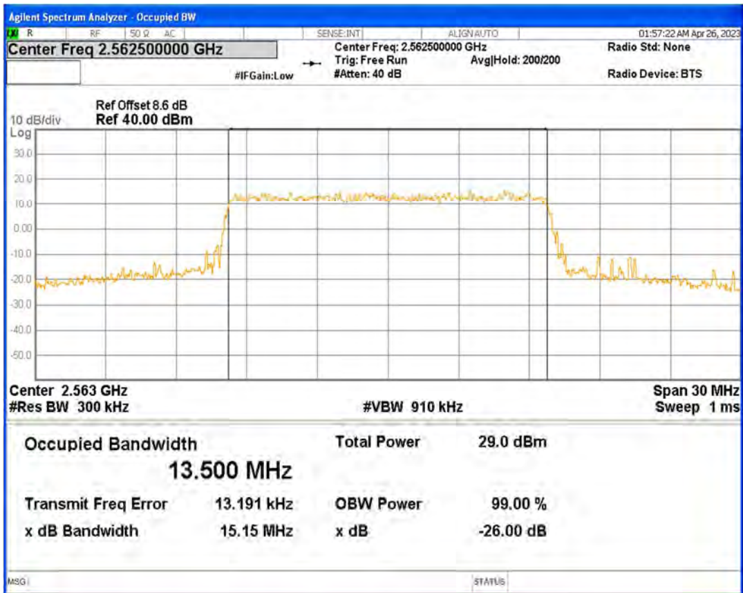
Band41(2555-2655) QPSK BW=15MHz Channel=40740 RB Size=75 Position=#0
