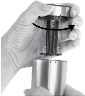
Insert 6 x AAA batteries into the removable cartridge. Ensure that the polarity of each battery follows the graphics.
