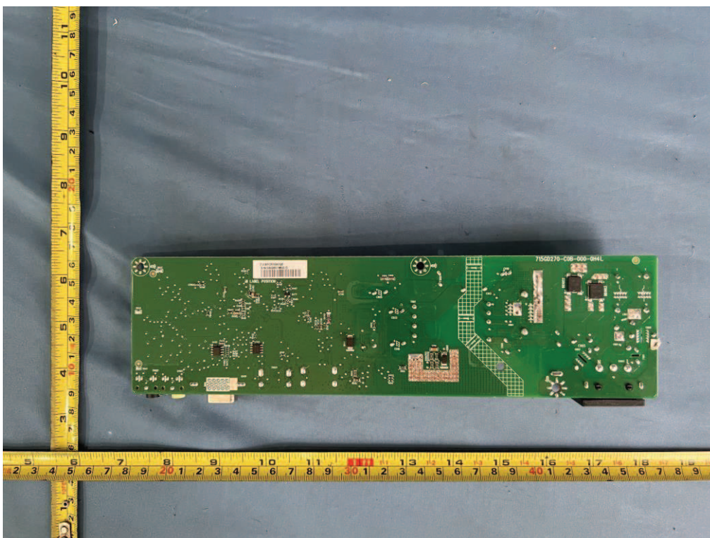
Figure 12. Power board 715GD270
