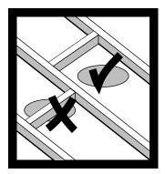
Determine position in ceiling where Fanlight is required to be installed. (Do not install within 120cm of stove or inside a shower recess). Be certain that the installation area is not restricted by roof beams above ceiling.
