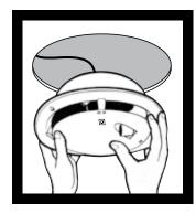
5. Remove light diffuser and air-intake grille. Unscrew the 3 screws on the lip of the unit until the gap between the toggles and inner lip of the unit is greater than the width of the Gyprock, or other ceiling material. Fold these toggles in. Push unit into hole.
