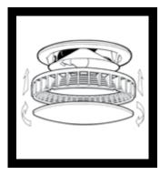
Push grille into unit and click into position. Assemble the diffuser and round dust seal and twist into position. To remove this assembly for cleaning, simply pull assembly downwards.
