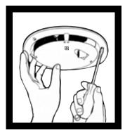
6. Turn the retention screws clockwise. The toggles will splay out. Tightening the retention screws allows the toggles to grip the ceiling material.
