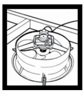
It is recommended that the three toggles be checked for the correct clamping by inspection from above. You may now insert a globe ≤ 75W into the R620 (not required for the R620LED)
