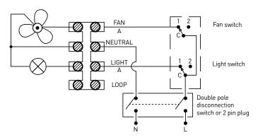
**Option 3:** Fan and light switched together with time delay on fan after switch is turned off
