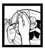
4. Remove terminal cover and wire according to the diagram in Option 1 over. This method of wiring switches fan and light on and off simultaneously. Option 2 shows how to wire fan and light separately. This allows the light (or the fan) to be switched on independently of the other. Option 3 shows the addition of a HPM Cat TX770/1RC time delay mechanism.
