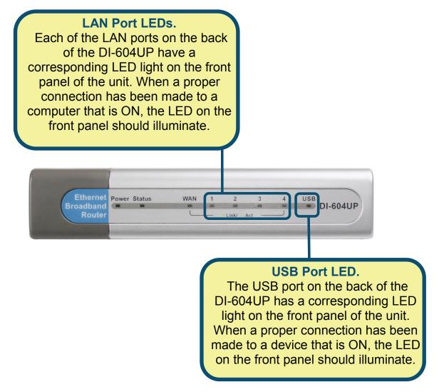
Additional printer may be added to your DI-604UP to increase functionality. By connecting a printer to the USB port at the back of the router, you may share print capabilities over your wired network. A valid USB connection will cause the corresponding USB LED at the front to light. For more information regarding USB connections and device implementation, see the DI-604UP user guide.
