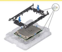
4. Align the processor with processor carrier by using your fingers to press the carrier on all the four sides until it clicks into place.
