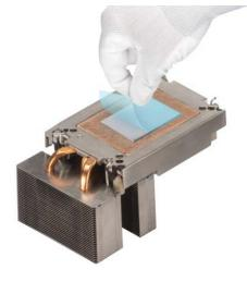
6. Place the heat sink on the processor and press the heat sink until the carrier locks onto the heat sink at all the four corners.
