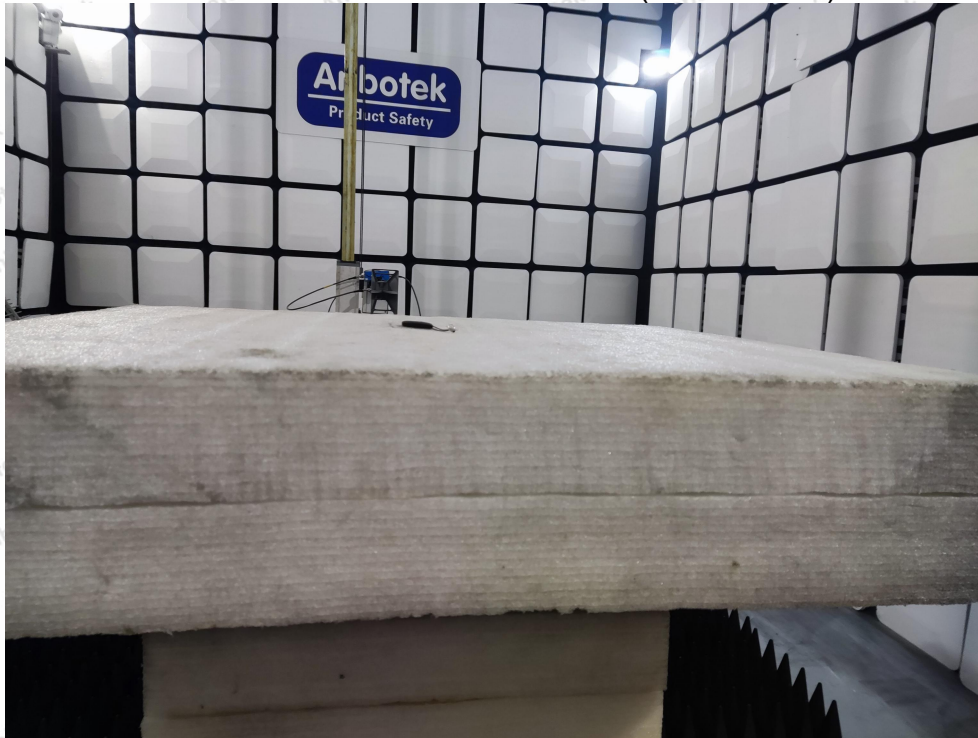
Photo of Radiation Emission Test (above 1GHz)
