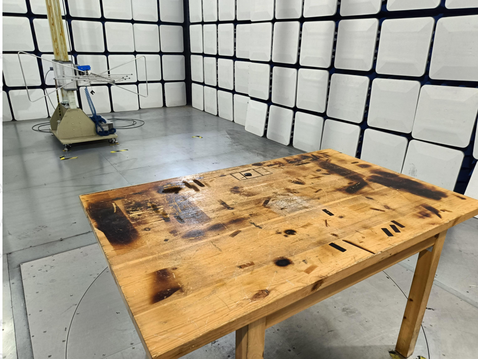
Photo of Radiation Emission Test (below 1GHz)
